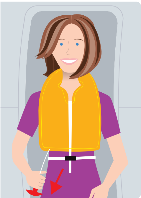
Pull red tag to inflate when exiting the aircraft
